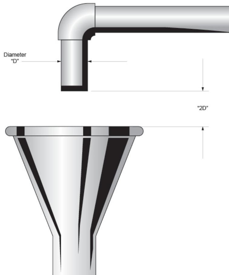
An air gap, although an extremely effective backflow preventer when used to prevent backsiphonage and backpressure conditions, may cause a corresponding loss of pressure to downstream outlets. Consequently, air gaps are primarily used at end of line services where reservoirs or storage tanks are desired.
