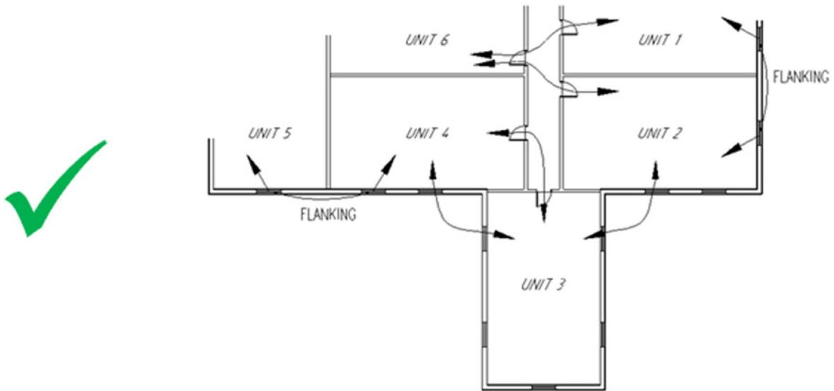
Figure 4 Example of layout planning - Bad acoustic practice to minimise flanking via external glazing and entrance doors, by not ensuring maximum distance between windows and doors.
