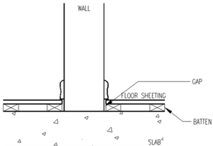
Figure 9 Floor lateral vibration isolation - Bad design practice
